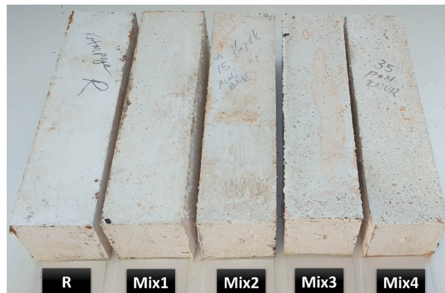
Fig. 3. The fabricated samples with different Hemp/PCM composites contents in gypsum matrix.
