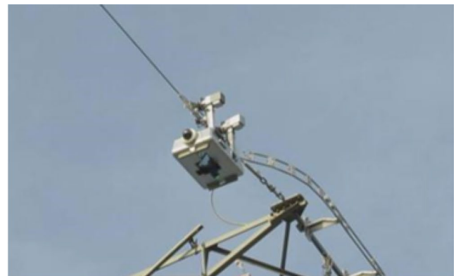
1. Driving arms; 2. Locking joints; 3. Grippers; 4. Battery control box; 5. Monitoring devices; 6. Driving wheel device; 7. Lifting device; 8. Guide device.
