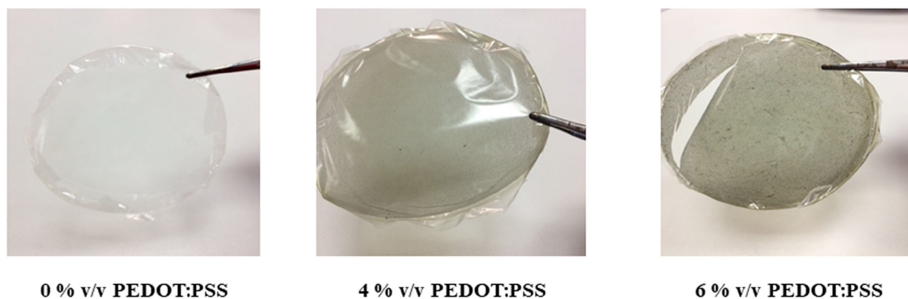
FIGURE 3 Images of fabricated polymeric films with different amount of PEDOT:PSS [Color figure can be viewed at wileyonlinelibrary.com ]
