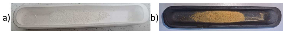
Fig. 5 – Photograph SnO 2 powder a) Before sulfuration b) After sulfuration at 500 °C for 24 h.
