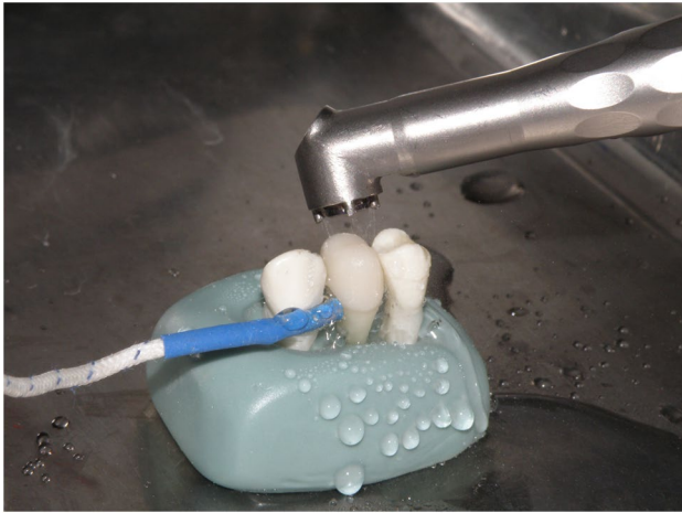
Fig. 2 Er:YAG laser irradiation of resin luted samples, aligned between the artificial tooth
