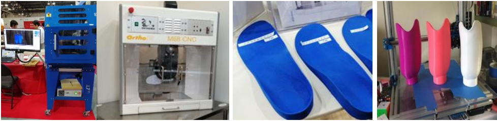
Fig.3. CAD and 3 D Printing is used for the other P&O.
