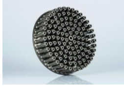
A 3D-printed injector head for Ariane 6 launcher [6]
