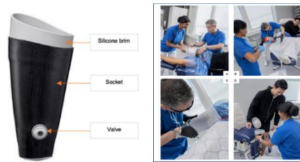
Fig.4. Direct socket (left) Direct socket process for TF amputee (right) A) application of material, B) resin injection, C) moulding of resin D) first fit and alignment check.
