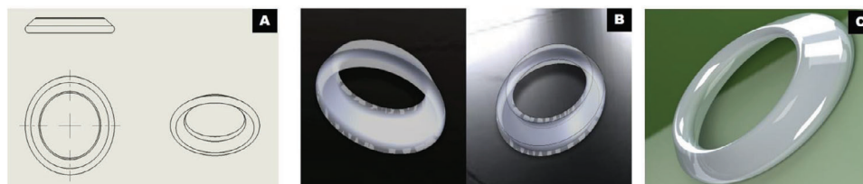
Figure 1. A) Simple design of the symblepharon ring, B) view of the inner and outer surfaces of the ring from different angles, and C) design of the 3D model.
