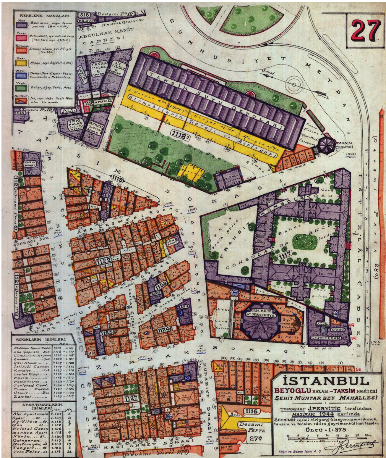
Figure 3. Pervititch insurance map, with legend designating construction techniques. Violet and pink colours indicate the use of RC (Ersoy and Anadol 2000).
