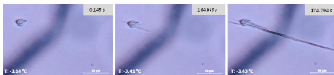
Figure 8. Morphology of an ice crystal grown in 40 % sucrose solution in the presence of 5 mg mL -1 \kappa -carrageenan and 1 mg mL -1 of AFGP.
