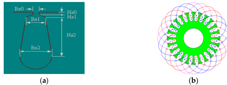
Figure 4. (a) Slot type of hub BLDC motor, and (b) double-layer winding connection.
