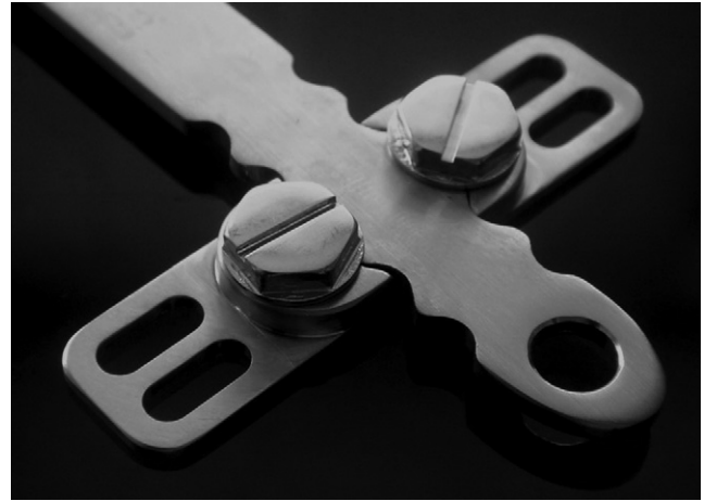
Fig. 2. Newly designed bar end with notches and screwed stabilizer.
