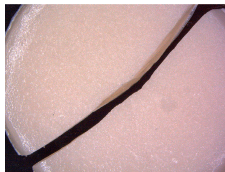
Fig. 3 Total fracture without delamination (8× magnification).
