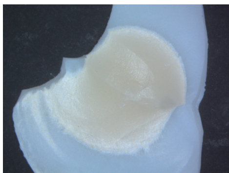
Fig. 2 Total fracture and a substantial level of partial delamination (8× magnification).
