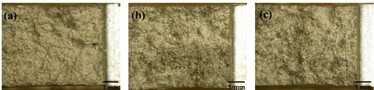
Figure 7. Fracture image of the sample at (a) 175 °C, 20x and (b) at 20 °C, 20x (c) at -75 °C 20x.
