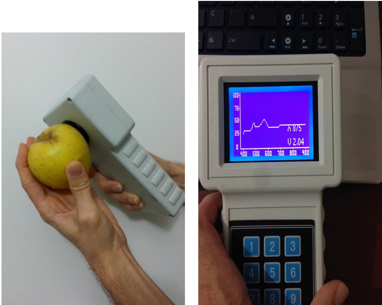
Figure 7. Use and operation of the proposed device: a) portable device and its use during measurement; b) graphical output of the measurement.
