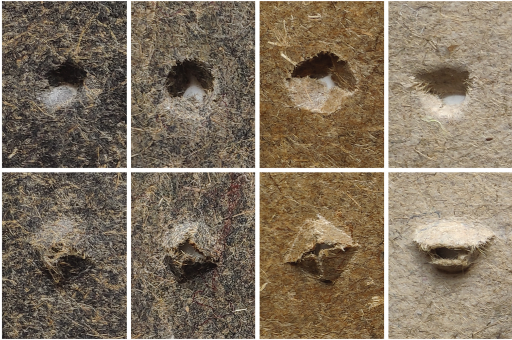
Figure 8. Entry and exit side damages of PPH, RPPH, PLAH, and LMPH from left to right.
