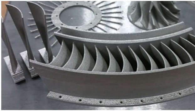
Fig. 1 Blisks, made of Inconel 718 with Additive Manufacturing [2]
