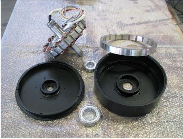
Figure 7. Stator with completed wound
