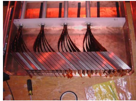
Figure 6.5: Photograph of the ZDC HAD section.
