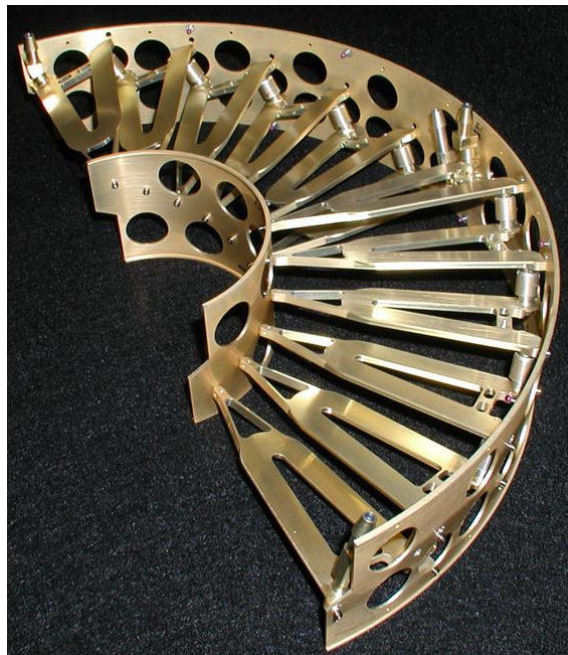
Figure 3.15: The FPix half-disk cooling channels mounted in the outer half-ring structure. The turbine-like geometry is apparent. Panels are mounted on both sides of the cooling channels.
