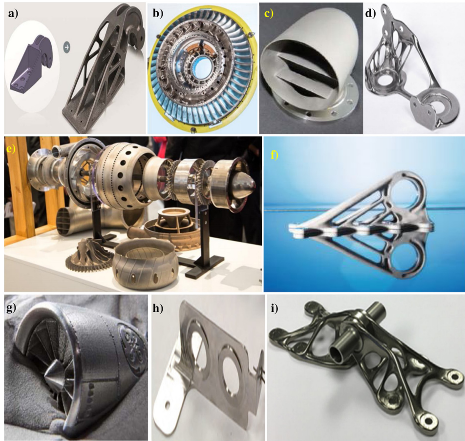
Fig. 5 – Aerospace components produced by AM technology: (a) Hing holder produced by Airbus with AM technology, (b) Rolls Royce Trent XWB engine manufactured with EBM method, (c) liquid oxygen flange produced by AM, (d) aerospace hinge part produced by laser powder bed method, (e) gas turbine engine by 3D printing, (f) bracket connector produced by Airbus, (g) leap engine fabricated with AM, (h) bald bracket manufactured by EBM, (i) complex shape Bracket designed with AM [69–76].
