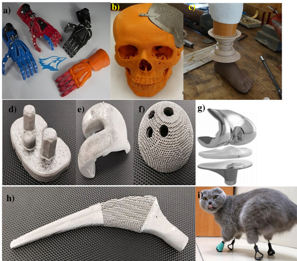
Fig. 7 – Medical applications using AM: (a) prosthetic hands in different colors, (b) cranial implant built with EBM, (c) a prosthesis socket produced with 3D printer for a little girl, (d) tibial tray produced by SLM, (e) femoral component, (f) acetabular cup built with 3D printer, (g) knee implant manufactured by AM, (h) hip stem manufactured by AM, (i) 4 Ti prosthesis was produced for a cat [88–96].
