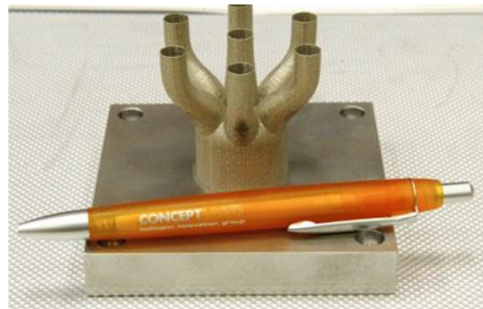
Figure 15. First test piece manufactured on M2 Cusing machine [6].
