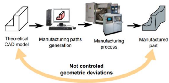
Figure 2. The usual numerical chain for Additive Manufacturing [4].
