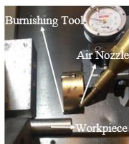
Fig. 1. Roller burnishing process in dry condition.
