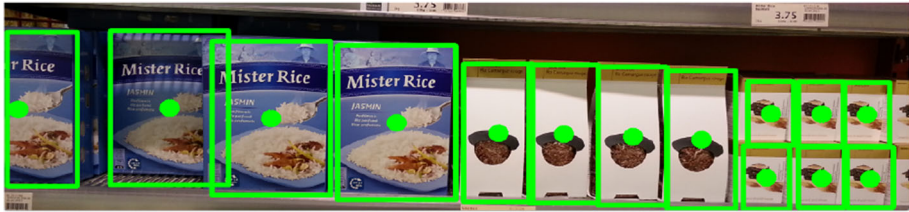
Fig. 10 Bounding box of the detected objects from the representative shelf image in the Grozi dataset with focused and iterative search
