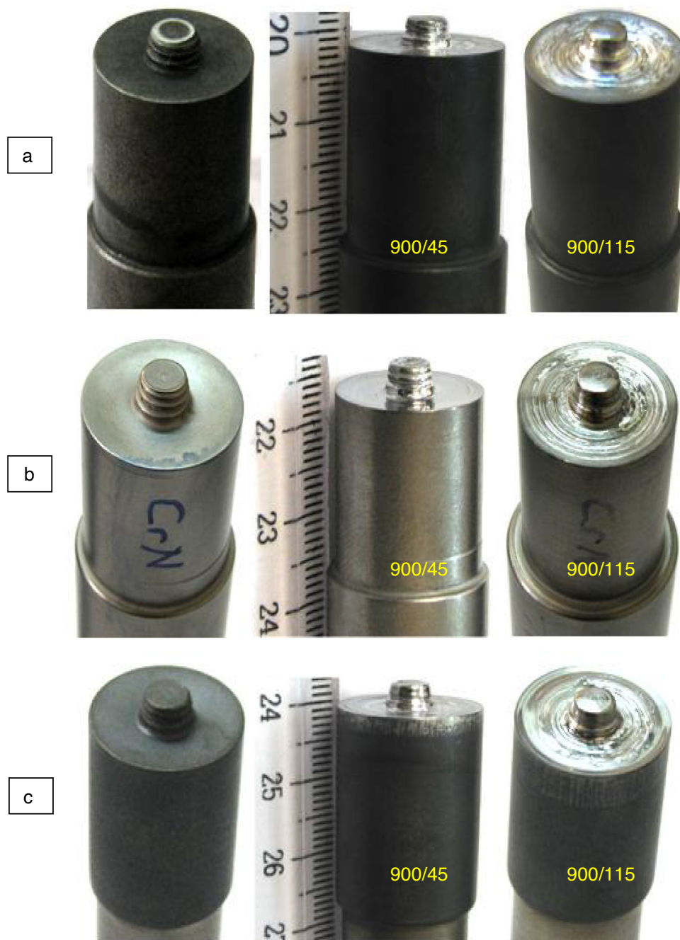
Fig. 6 – Macrographic views of: (a) uncoated tool, (b) CrN coated tool, (c) AlTiN coated tool before and after welding process.
