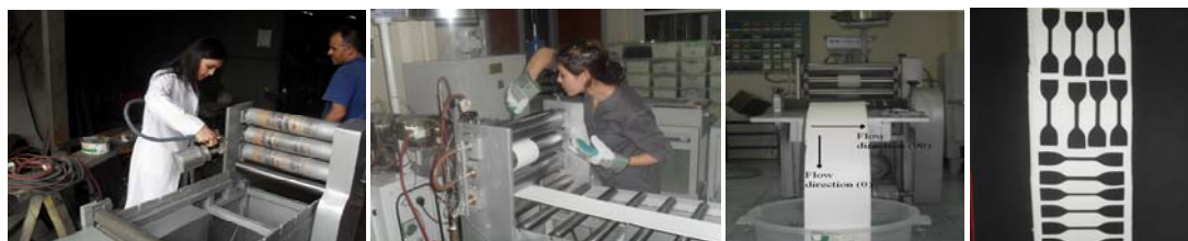
Fig. 1. Plate machine, extruder head and flow directions
