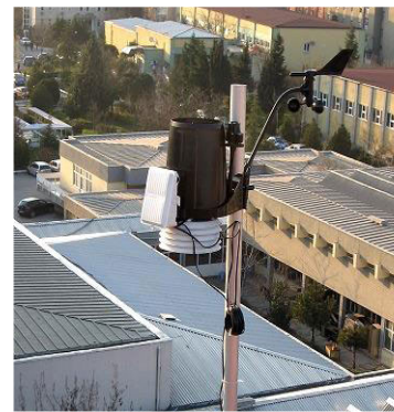
FIGURE 12. Weather station on the rooftop of laboratory building for meteorological data utilization.
