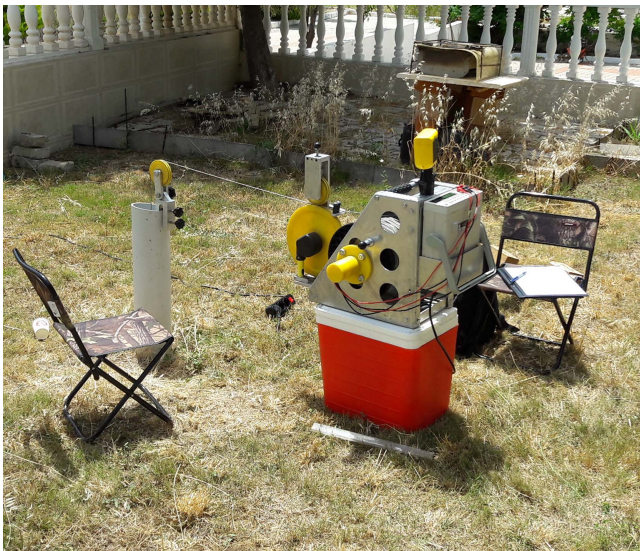
Figure 5. General view of the T–D logging system.
