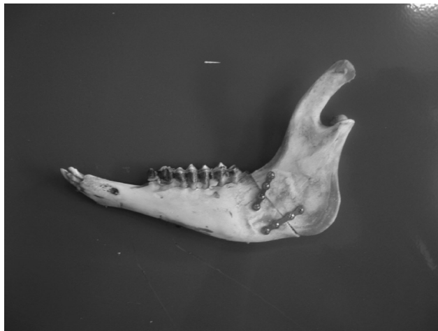
Fig 5 Group B: biplanar dual-miniplate, upper border-proximal 3 holes bicortical fourth hole monocortical, lower border-bicortical.
