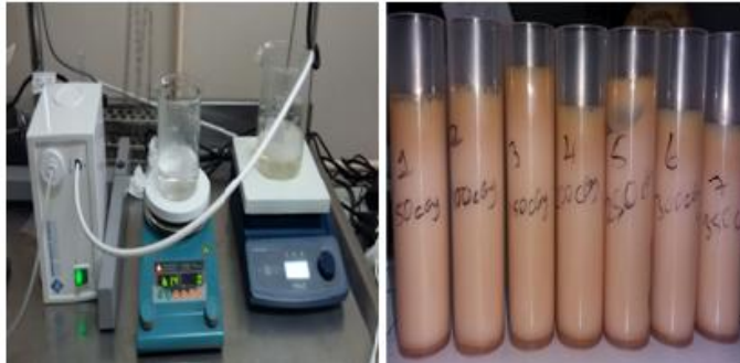
Figure 1. a) gel production assembly, b) the samples (after irradiation).
